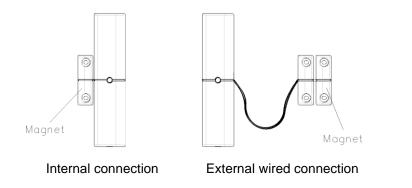
Choose either the internal or external wired connection, both of which types cannot be in existence at the same time.
